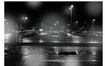
IR reflection and smudges cause image distortion
