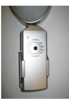
Fig.8 Walk-Tester in holder and fitted to detectors, ready for walk testing
