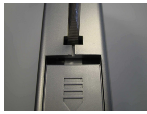
Fig.3. Removing battery compartment cover
