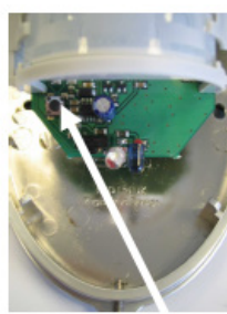
Fig.7. Detector's programming button
